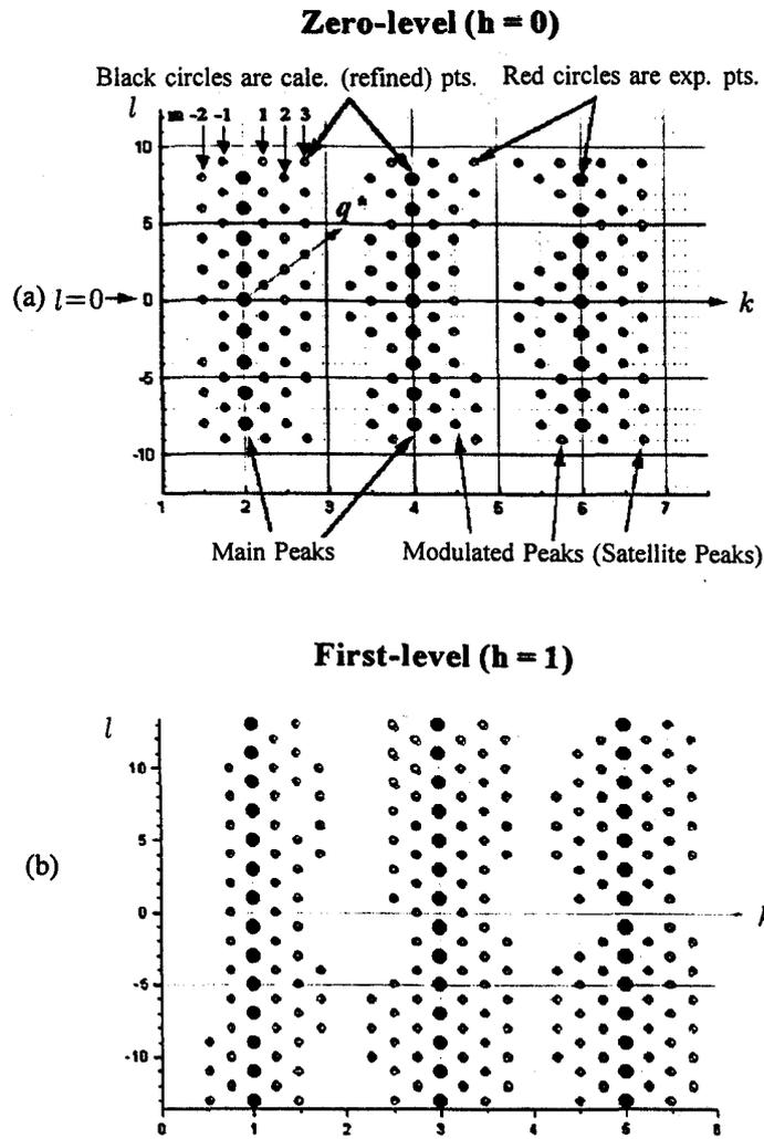
FIG. 9. Plot of reflection points in reciprocal lattice space. The larger circles are the main reflections; smaller circles are the satellite reflections.  $m$  is the fourth component of scattering vector  $\mathbf{Q}(h, k, l, m)$ .
