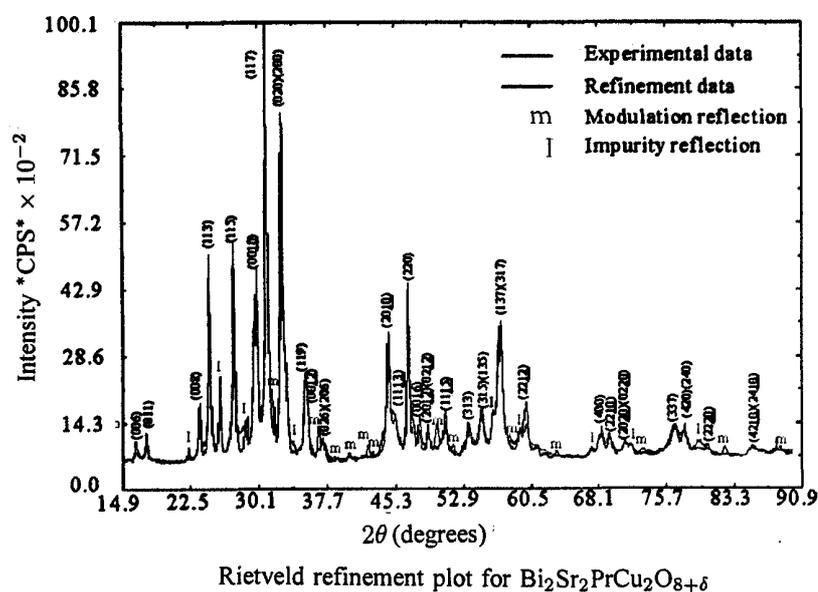
FIG. 2. X-ray diffraction pattern with peak index of main phase (Pr-doped Bi2212) labeled. Bold line is plotted with experimental points ( $\theta/2\theta$  scan in  $0.01^\circ/0.02^\circ$  step). Thin line is the calculated curve take into account the contribution of Pr-doped Bi22 12, Bi2201,  $\text{Bi}_2\text{O}_3$  and  $\text{SrO}_2$  phases.
