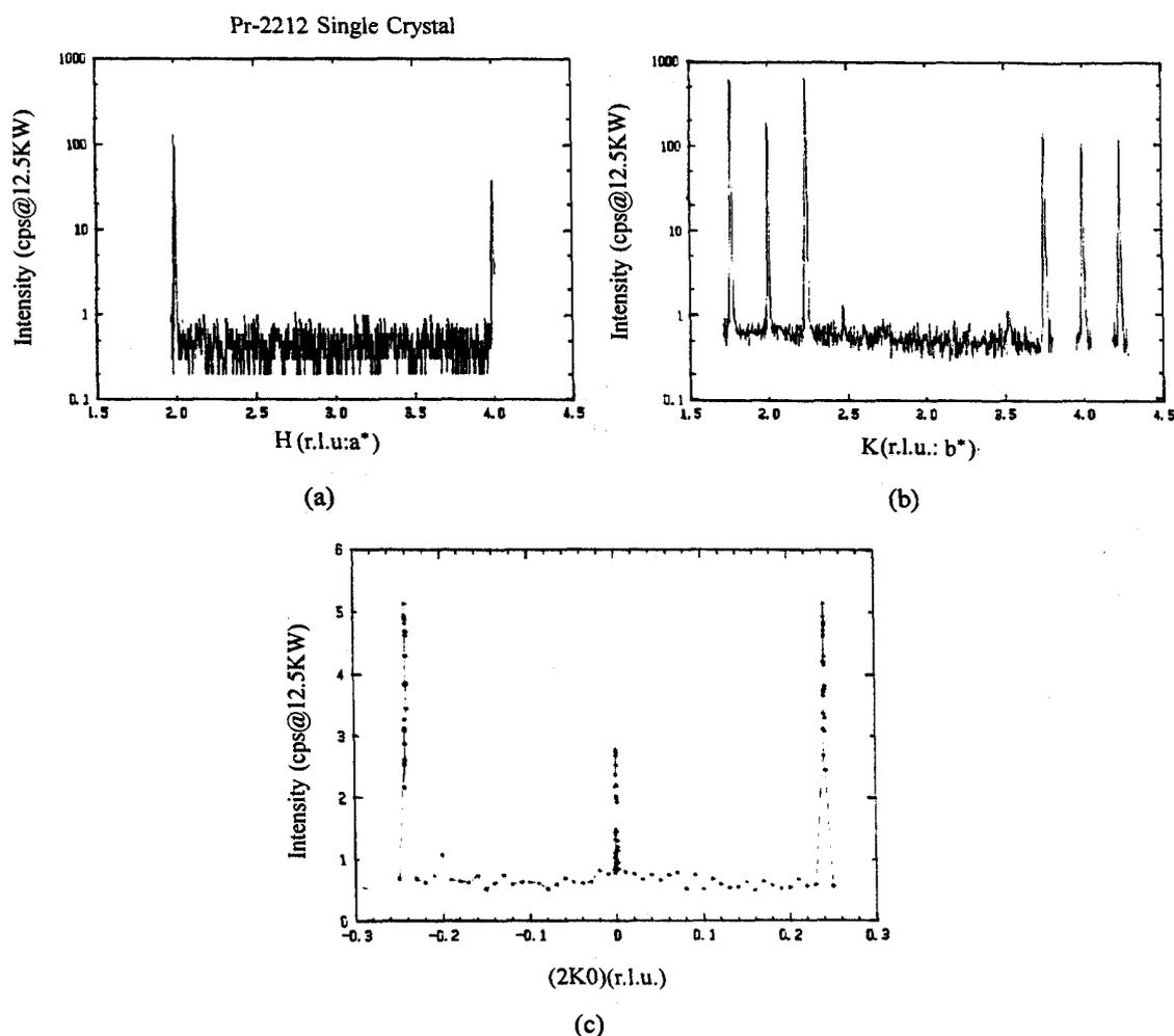
FIG. 4. Plane GIXD diffraction pattern of a small  $\text{Bi}_2\text{Sr}_2\text{PrCu}_2\text{O}_{8+\delta}$  single crystal ( $\sim 6 \times 4 \times 0.15 \text{ mm}^3$  in size). (a) GIXD scan along (H00) direction. (b) GIXD scan along (0K0) direction. (c) GIXD scan along (2K0) direction.
