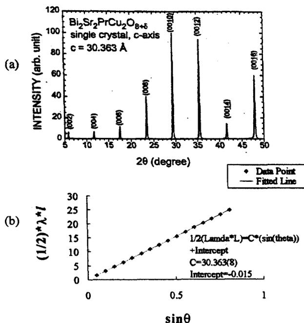
FIG. 3. (a) Diffraction patterns of  $\theta/2\theta$  scan of a single crystal along  $c$ -axis, using a crystal of size  $\sim 5 \times 4 \times 0.04 \text{ mm}^3$  with  $ab$  plane on a low background quartz plate ( $6^\circ$  off cut the (0002) plane). (b) Plot of  $(\lambda/2 \cdot l)$  vs.  $\sin\theta$  for determination of  $c$ -axial length.
